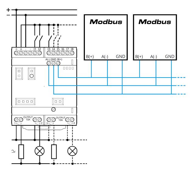
Modbus RTU wiring diagram using the RS-485 interface
